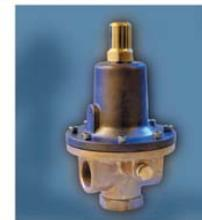
REGO's BR-1780 series regulators are specifically designed for final-line pressure regulation for hospital oxygen systems. Equally suitable for variety of gases in medical or industrial applications. Balanced seat design provides constant delivery pressure ranges (5-55psig, 40-110psig, 100-200psig) with varying inlet pressures (up to 400 psig) and wide range of flow demand. Temperature range -40°F to 165°F. Flow rates up to 16,000 SCFH.
